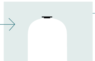
Welding of boss to liner
