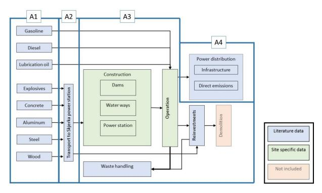
**Error! Reference source not found.** shows the structure of the LCA-model. It illustrates which life cycle stages that are included and whether the data used is generic or specific.
