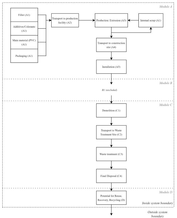
Modules A1-A5 and C1-D are included. The figure below shows a (simplified) process tree.
