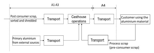
Fig. 2 Flow sheet for modules A1 – A4 for 1 kg of aluminium extrusion ingot from aluminium recycling plant.
