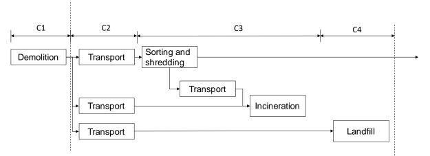
Fig. 3 Flow sheet for modules C1 – C4 for 1 of aluminium extrusion ingot after end of useful life. C1 is included but
