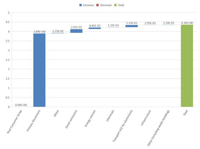
*Fig. 1 A waterflow diagram showing the contributions to climate change (GWP-Total in kg CO*<sub>2</sub>/*kg Al) for Azuqueca for modules A1-A3.*
