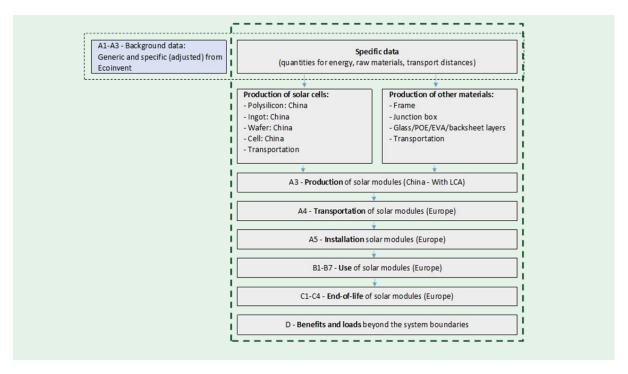
The PolySi, ingots, wafers, cells and modules are manufactured in China. The supply chain is shown below:
